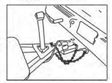
Properly mounted safety chains. Note that the jack is fully raised and dolly wheel removed.
