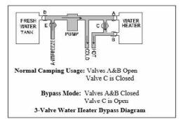
**NOTE:** In the 3-valve bypass diagram, valve D is the fresh water tank shutoff. Valve E is used to introduce RV antifreeze into the lines when winterizing the system and has a clear hose attached to it. See Winterizing the Plumbing System. Valves D and E are typically located near the water pump, which may be under a dinette bench, kitchen island, or bed.
