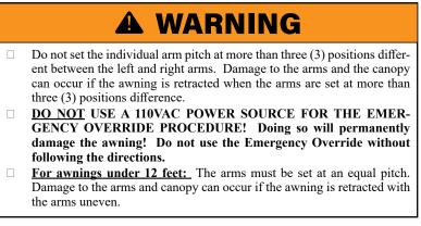
The longitude arms have 6 pitch adjustment settings. The awning can be extended and retracted in any of these positions without resetting the pitch.
