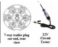
The connector plug may build up corrosion with extended use. It should be cleaned periodically to insure good electrical contact. Make sure the connector plug is kept clean and protected from road elements as you travel.
