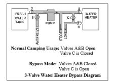
**NOTE:** In the 3-valve bypass diagram, valve D is the fresh water tank shutoff. Valve E is used to introduce RV antifreeze into the lines when winterizing the system and has a clear hose attached to it. See Winterizing the Plumbing System. Valves D and E are typically located near the water pump, which may be under a dinette bench, kitchen island, or bed.
