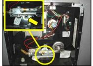
Water Heater Drain Plug Location
