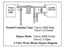
**NOTE:** In the 3-valve bypass diagram, valve D is the fresh water tank shutoff. Valve E is used to introduce RV antifreeze into the lines when winterizing the system and has a clear hose attached to it. See Winterizing the Plumbing System. Valves D and E are typically located near the water pump, which may be under a dinette bench, kitchen island, or bed.
