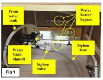
Water valves and water heater bypass
