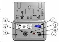
Fresh Water Connection inlet at the utility center should be unplugged (i.e., the non-toxic drinking water hose disconnected) when the recreation vehicle is unattended for any amount of time. If something would happen to the water system, this may help limit water damage to a smaller area.
