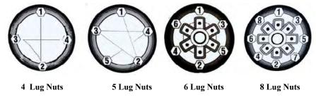
Criss cross "star" patterns, as shown, must be followed during tightening sequence
