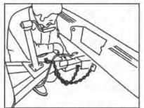
Repeat Step 2 with right chain. Slack for each length should be the same but not more than necessary to permit the vehicle to turn at the minimum radius.
