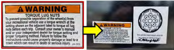
Lug nut torque pattern and warning label
