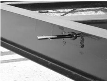
**Fig. 1-Through Frame Crank Extension w/pin**
