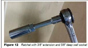
Figure 12 Ratchet with 3/8" extension and 5/8" deep well socket
