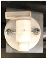
Exterior Fresh Water Drain Example
