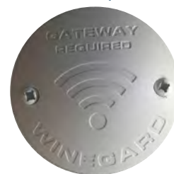
Wi-Fi Prep Location (Found on Ceiling of RV)
