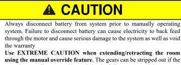
□ Use EXTREME CAUTION when extending/retracting the room using the manual override feature. The gears can be stripped out if the room is manually retracted/extended to its fullest extent and the operator continues to rotate manual override. Damage can also occur to the slide components, slide room structure or trim components. Damages due to misuse of the manual override feature will void any and all claims to the Limited Warranty.
