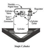
right hand swivel nut to the cylinder valve. Secure the cylinder to the A-frame bracket using the bolts, nuts and washers provided. 7.
