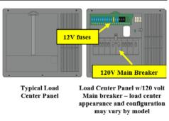
Motor homes may have separate small panels for breakers and fuses. They
