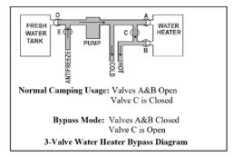
**NOTE:** In the 3-valve bypass diagram, valve D is the fresh water tank shutoff. Valve E is used to introduce RV antifreeze into the lines when winterizing the system and has a clear hose attached to it. See Winterizing the Plumbing System. Valves D & E are typically located near the water pump, which may be under a dinette bench, kitchen island, or bed.
