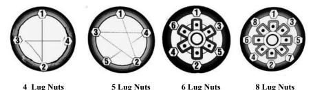
Criss cross "star" patterns, as shown, must be followed during tightening sequence
