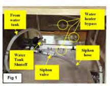
Water valves and water heater bypass
