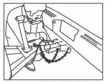
Repeat Step 2 with right chain. Slack for each length should be the same but not more than necessary to permit the vehicle to turn at the minimum radius.
