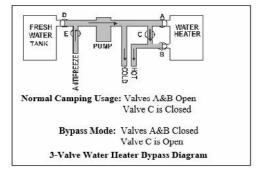
**NOTE:** In the 3-valve bypass diagram, valve D is the fresh water tank shutoff. Valve E is used to introduce RV antifreeze into the lines when winterizing the system and has a clear hose attached to it. See Winterizing the Plumbing System. Valves D and E are typically located near the water pump, which may be under a dinette bench, kitchen island, or bed.
